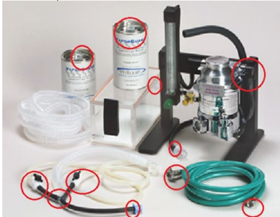
Attachment 4: Common places for WAG leaks
