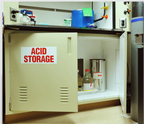
Store acid in a ventilated corrosive cabinet
