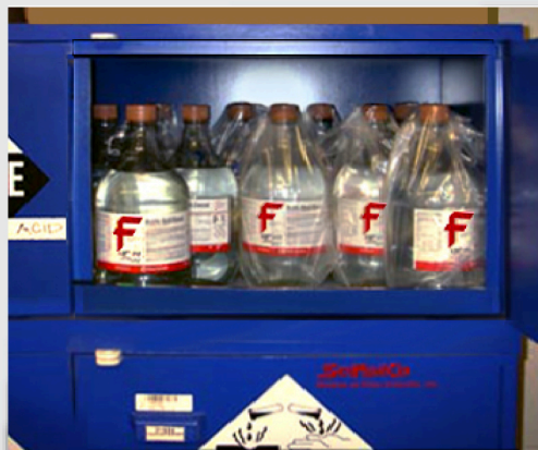
Store bases in a corrosive cabinet
