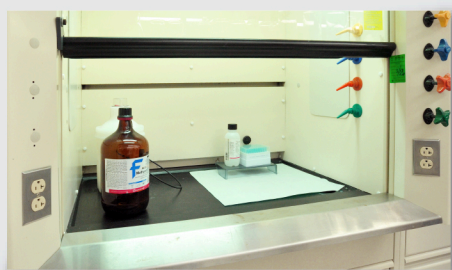
Engineering Control: Chemical Fume Hood
