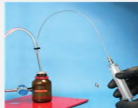
Fig. 1. Filling syringe using inert gas pressure. Image form Aldrich Tech Buletting AL-134
