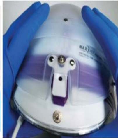
3C: Pull Filter Cover Cap fully down on the helmet by squeezing in a downward motion, aligning the T-Tab hole (A) with the helmet rear bottom snap (B)
