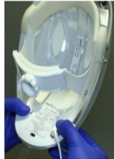
4C: Secure the two bottom snaps
