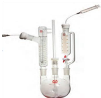
Fig 2. Syringe transfer of reagent to reaction flask. Image from Aldrich Technical Bulletin AL-134
