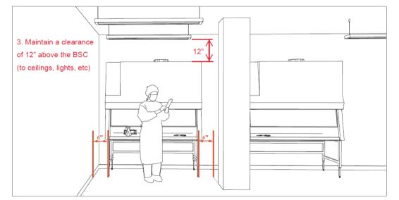
4. Maintain a clearance of 6" on sides and behind the BSC (to walls, columns, benchtops, equipment, etc)
