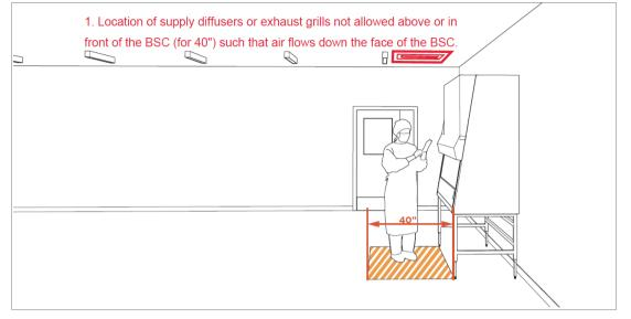
2. Maintain an undisturbed space of 40" around the BSC. \*Undisturbed means free of both permanent (walls, cabinets, equipment) and temporary (door swings, people traffic, cabinet drawers/doors) encroachment.
