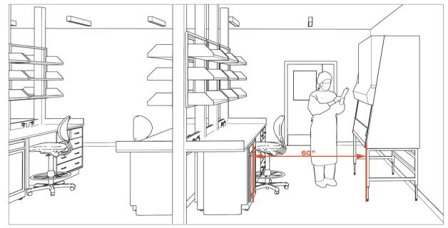
Maintain a clearance of 60" in front of the BSC if there is any possibility of traffic behind the occupant working at the BSC.
